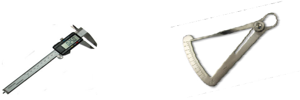
Calipers used to measure thickness of an item
